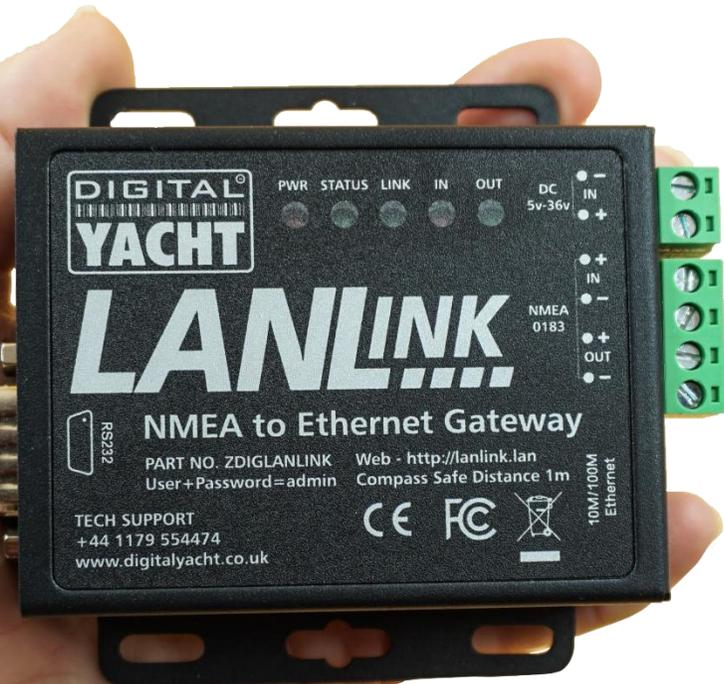
LANLink is available in two versions suitable for NMEA 0183 and NMEA 2000 respectively. It features an easy to use web interface allowing any device with a browser to configure NMEA baud rates and IP/Port information.
